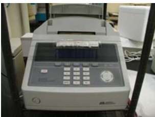
Name: PCR Thermal cycler Type: Applied Biosystems GeneAmp PCR System 9700 Location: Analysis Room
