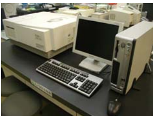
Name: Spectrofluorophotometer Type: Shimadzu RF-5300PC Location: Analysis Room
