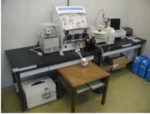
Name: Autoanalyzer Type: BL-TEC Autoanalyzer QuAAtro2-HR (4ch) Location: Analysis Room
