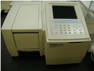
Name: UV-Vis Spectrophotometer Type: Shimadzu BioSpec-mini Location: Analysis Room
