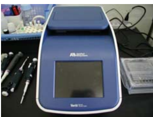
Name: PCR Thermal cycler Type: Applied Biosystems Veriti 96-well Thermal Cycler Location: Analysis Room
